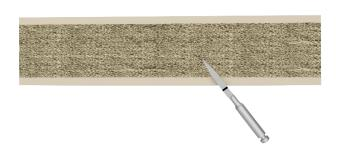
Step 3: Drill to depth using a 2 mm twist drill.
