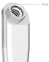
Figur 21: Hak i implantat hex.
