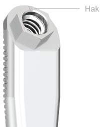
Figur 21: Hak i implantat hex.
