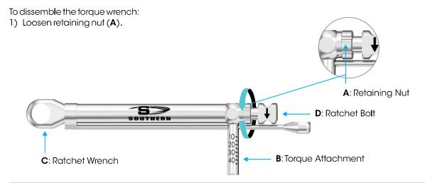
2) Slide the ratchet bolt (**D**) out of the ratchet wrench (**C**).
