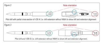
The orientations indicated in Figure 2 and Figure 3 ensure that the catch feature of the drill extension (circled in blue) slots into the latch groove of the drill (circled in green). This prevents the drill from sliding out of the drill extension.
